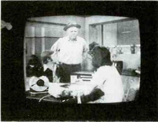
These photographs show a simulated comparison between analog and digital video at a poor 4-dB signal-to-noise ratio.
