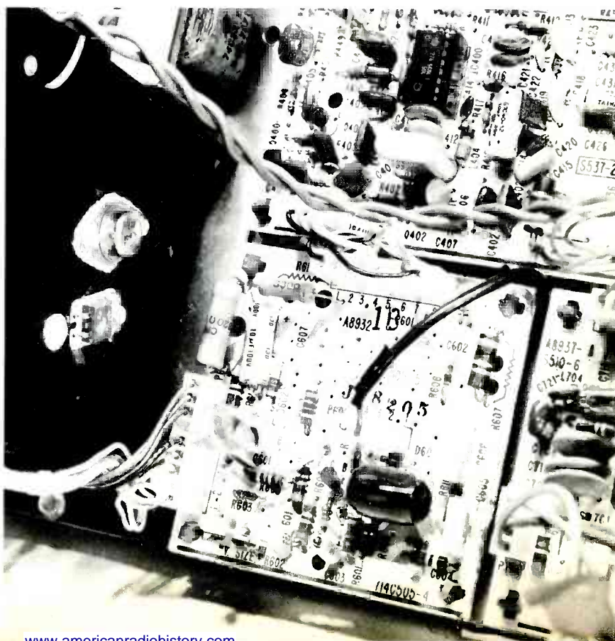
Fig. 1 Most of the vertical-sweep components of the Admiral M24 and M25 chassis are mounted on the M600 module. The output transistors and associated resistors are located on the large flat heat sink.
