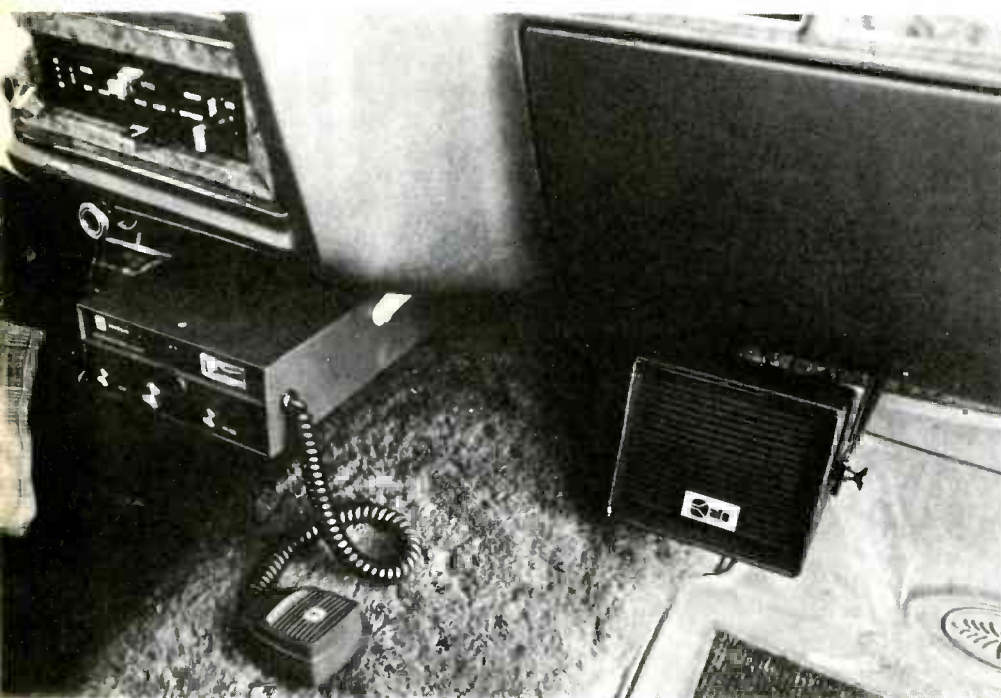
Fig. A "KRIKET" Model 3035 external speaker and a CB transceiver were mounted in a car for listening and frequency-response tests.
